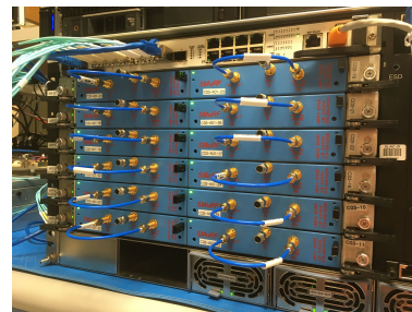
Room temperature SMuRF Electronics. Generate + digitize probe tones and apply amplifier, squid, and detector biases (designed + fabricated at SLAC)
