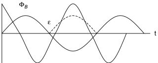
If the slip rings are replaced by a commulator, the path in dotted lines is followed.
