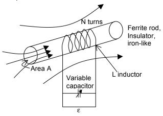
An LC resonant circuit is formed with  $Q \approx 100$
