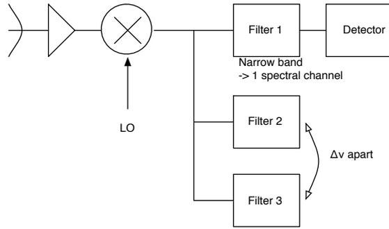
Measure a single channel. The filter has a bandwidth  $\Delta\nu$ . Step the local oscillator in steps of  $\Delta\nu$  to change the frequency that is being looked at.
