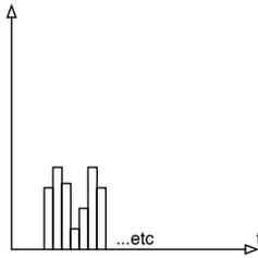
Add additional filters and detectors to detect multiple spectral lines simultaneously using a single radio telescope. Called a "filter bank". Gets very complex when you're wanting to observe many frequencies.
