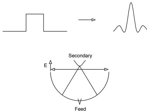
For a radio telescope, the aperture distribution is the [electric] field (both amplitude and phase) across the front of the dish.
