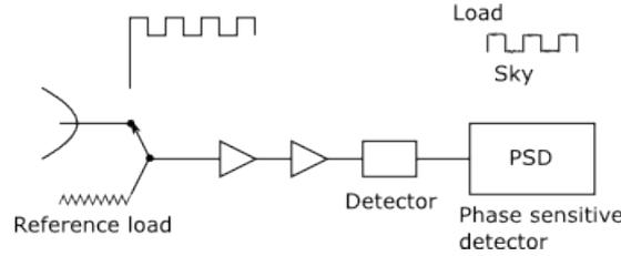
PSD gives  $\propto (T_A - T_{load})$ . Want to arrange the sky and the load temperatures so that they are as close as possible together.
