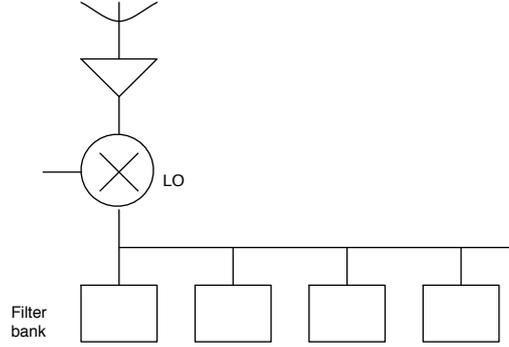
Nowadays digitize the full band as it comes out of the mixer, and do the dispersion correction in software. Known as Coherent De-dispersion. Essentially a software receiver. Multiply the digital signal by the inverse of the dispersion transfer function.
