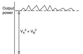
Any gain fluctuations in either A or B will modulate the DC component up or down, increasing the difficulty of measuring the fringe pattern.
