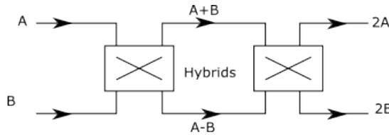
The outputs A and B have identical gain fluctuations. Hence the difference  $2A - 2B$  is free of  $\frac{1}{f}$ . It also cancels the atmospheric fluctuations.
