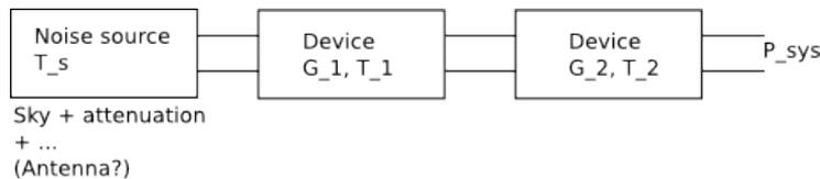
NB:  $T_1, T_2$  are the noise temperatures, not the actual temperatures.
