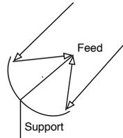
Prime focus - simple, just one reflecting surface. Difficult to feed, as the feed is not very far from the dish surface, so power needs to be collected from a wide spread of angles. Also means that the feed will see some power from over the edge of the dish - the ground, which can produce a large amount of noise. Lowish maximum efficiency, less than around 60%.
