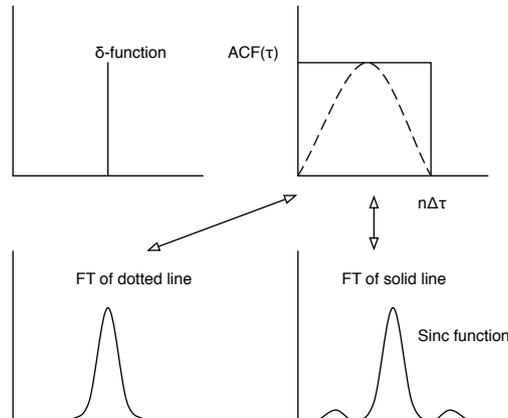
How close the spike is to a delta function depends on the number of delays that we measure. But get sidelobes (sinc function). This becomes a problem if we have two lines close together, then the sinc functions overlap and things start to get confusing. By choosing the window  $f^n$  (weight the ACF [dashed line]) we suppress the sidelobes, and degrade the resolution. This is normally acceptable. Normally use a  $\cos^2$  weighting function.
