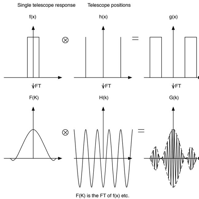
The fringe pattern is limited by the size of the individual dishes, while fringe separation is determined by the separation of the elements.
