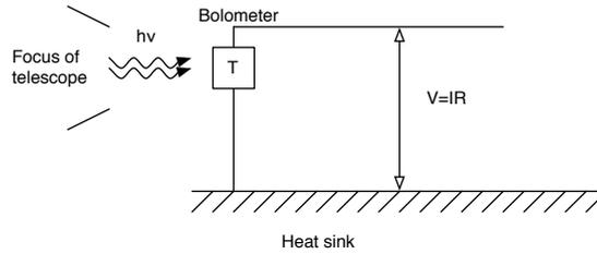
A dc bias is applied. Photons are absorbed  $\rightarrow$  the temperature rises  $\Rightarrow V$  changes and is amplified. The heatsink is present to cool the bolometer down as quickly as possible once it's received some energy.
