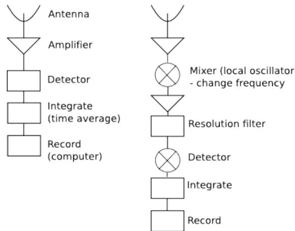
Most receiver systems, especially for spectral line, pulsars and interferometry, have a mixer or down-converter which changes the frequency of the signal. Why?
