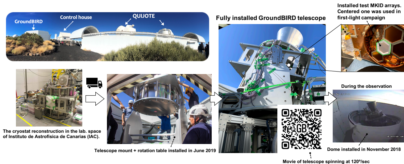
Figure 5: Installation of the GroundBIRD telescope. One of the enclosed spaces originally for the Very Small Array experiment is now used for GroundBIRD, as shown in the photo at the top left. The cryostat chamber was installed in the Teide observatory following the reconstruction and cooling test at the laboratory space of the IAC. The movie of the telescope rotating at 120°/s can be accessed via the QR code ( https://photos.app.goo.gl/ivjrhVkwJcSDzahNA ).
