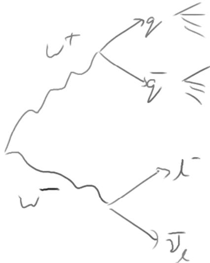
Identify particles to jets, and measure the invariant mass of the di-jet system. This should be the mass of the  $W^+$ . The lepton is easy to detect, and the neutrino can be deduced through missing momentum and energy. Can hence reconstruct the  $W^-$ . Combined with the  $W^+$ , we can measure all of the components of the interaction.
